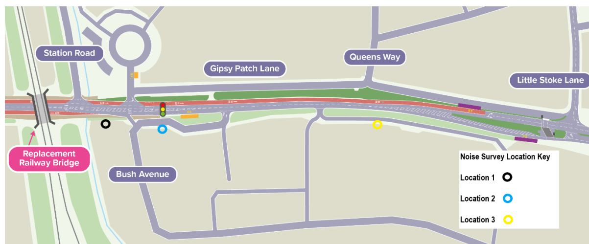
FIGURE 1: NOISE MONITORING LOCATIONS
